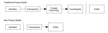
As an additional firewall, a new key pair should be used for each transaction to keep them from being linked to a common owner. Some linking is still unavoidable with multi-input transactions, which necessarily reveal that their inputs were owned by the same owner. The risk is that if the owner of a key is revealed, linking could reveal other transactions that belonged to the same owner.
